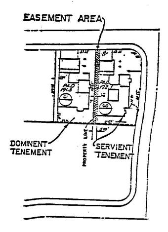
This sketch indicates the location of the five foot (5') sideyard easement described herein, and the designation of dominent and servient tenements and property line. All other measurements, figure, and references appearing thereon are purely for illustrative purposes and do not necessarily represent actual measurements and actual data pertaining to the real property described herein.
