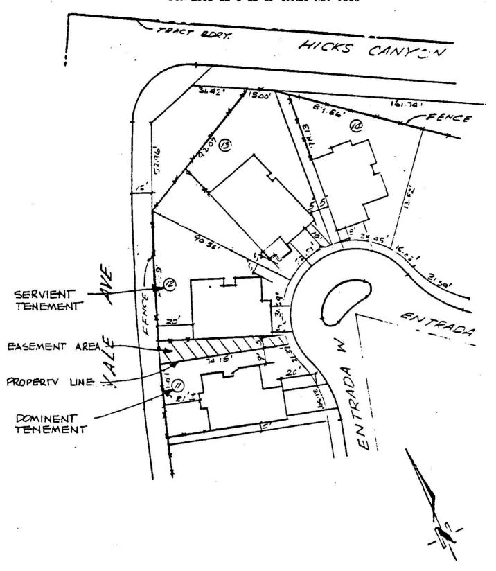
This sketch indicates the location of the sideyard easement and the designation of the dominent and servient tenements as related to property line. All other measurements, figures, and references appearing hereon are purely for illustrative purposes and do not necessarily represent actual measurements and actual data pertaining to the property described hereon.
