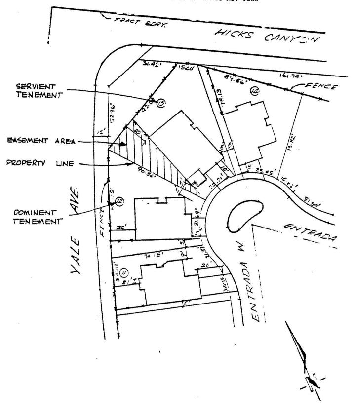
This sketch indicates the location of the sideyard easement and the designation of the dominent and servient tenements as related to property line. All other measurements, figures, and references appearing hereon are purely for illustrative purposes and do not necessarily represent actural measurements and actual data pertaining to the property described hereon.
